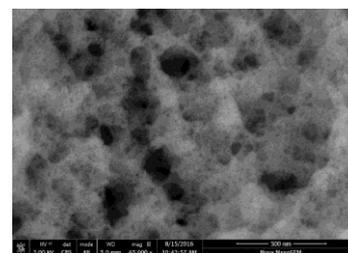
Figure 3. Silica hydrogel matrix (SEM)
