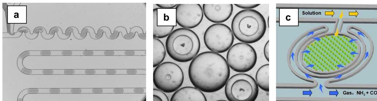
(a) Droplets created in a microfluidic system and (b) crystals in double emulsions and (c) the crystal hotel
