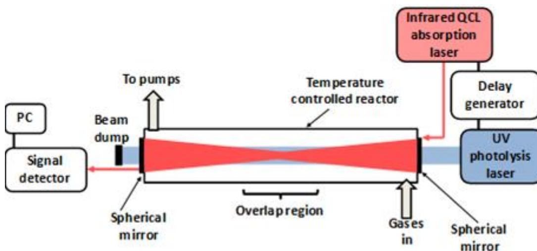
Figure 2: Schematic of experimental apparatus for infrared absorption measurements of Criegee intermediates and reaction products.
